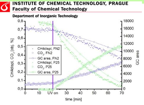
Tests of hexane degradation in the FN2 ® paint on the roof bag.
